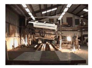
The image above depicts the fixture used to conduct roof crush dynamic testing in a testing laboratory in Salinas, California. The road surface moves along the track, contacting the roof of the vehicle as it rotates on the spit. The test surface impacts both *sides of the roof on a single run*, imitating the first roll of a vehicle in a rollover crash. The picture shows a 1994 Chevrolet Suburban (*vehicle in white*).
