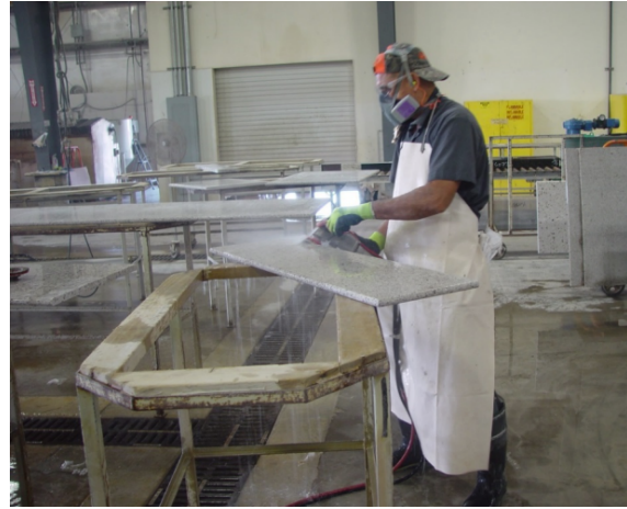
Left: Stoneworker cutting stone using a dry method (source: Washington State Labor & Industries). Right: Stoneworker using a wet grinder and respiratory protection (source: Centers for Disease Control and Prevention).
