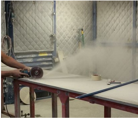
Left: Stoneworker cutting stone using a dry method (source: Washington State Labor & Industries). Right: Stoneworker using a wet grinder and respiratory protection (source: Centers for Disease Control and Prevention).
