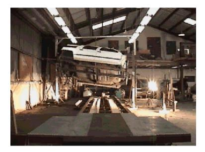
The image above depicts the fixture used to conduct roof crush dynamic testing in a testing laboratory in Salinas, California. The roadway surface moves forward along the track, contacting the roof of the vehicle as it rotates on the spit. The test surface impacts both *sides of the roof a single time*, imitating the first roll of a vehicle in a rollover crash, with repeatable results. The picture shows a 1994 Chevrolet Suburban with two dummies inside.
