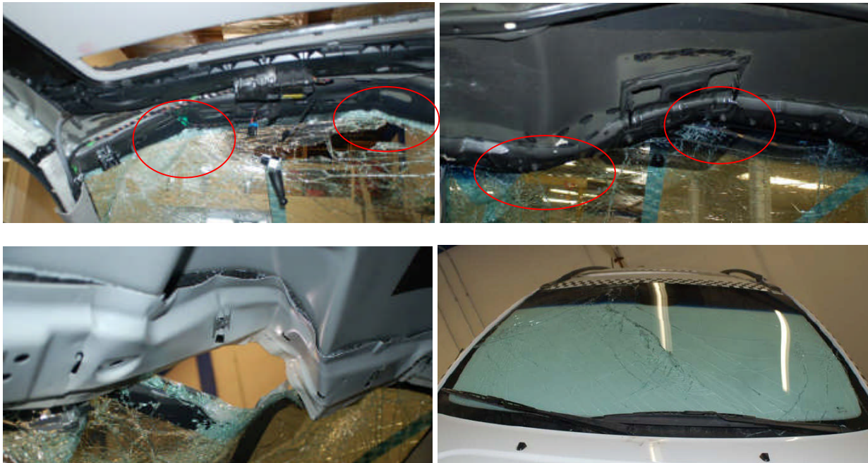
Figure 6. Interior views of the Jetta (above left) and Camry (above right) show buckled windshield headers after the second roll test. The G6 (below left) windshield header performed particularly poorly. The Volvo XC90, after two roll tests at 5° pitch on the JRS (below right), shows no structural failures.
