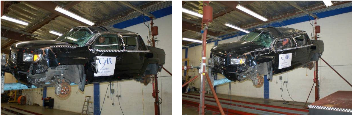
Figure B1. The Honda Ridgeline after first (left) and second roll JRS tests.
