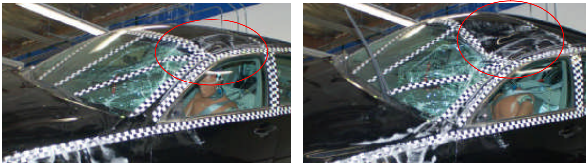
Figure 1. Photographs of a 2007 Toyota Camry roof after one roll and after two rolls in a JRS test showing the buckling of the windshield header in this vehicle. The Toyota Corolla showed similar buckling in a JRS test.
