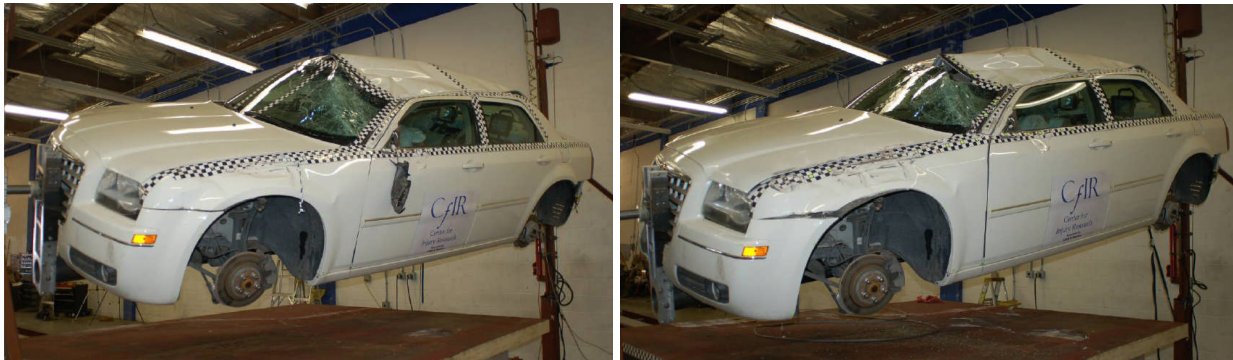
Figure 2. The 2006 Chrysler 300 after the first JRS roll test (left) and second roll.
