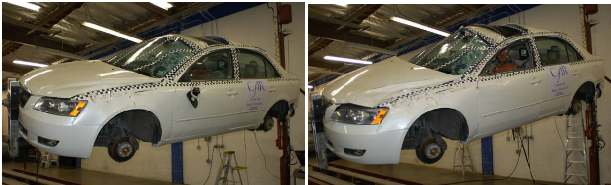
Figure 3. The 2006 Hyundai Sonata after the first JRS roll test (left) and second roll.
