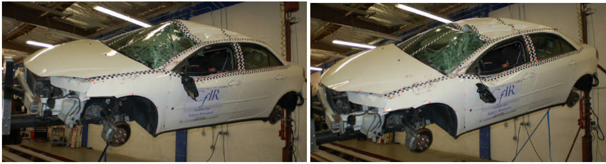
Figure 1. Pontiac G6 after first (left) and second roll JRS tests.
