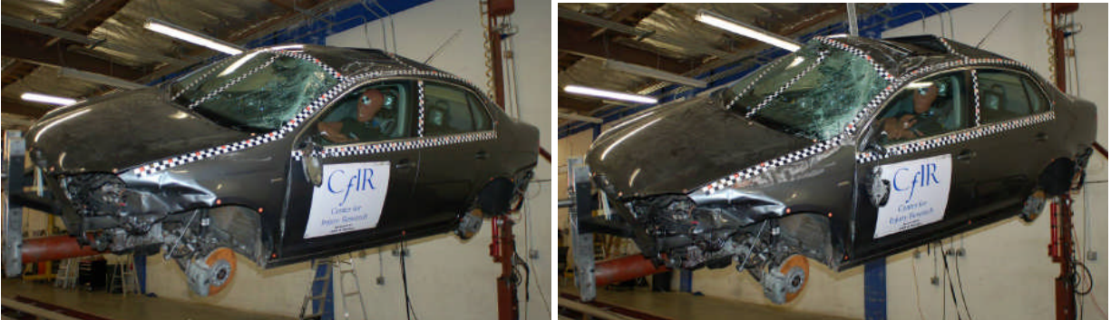
Figure 5. Volkswagen Jetta after first (left) and second roll JRS tests.
