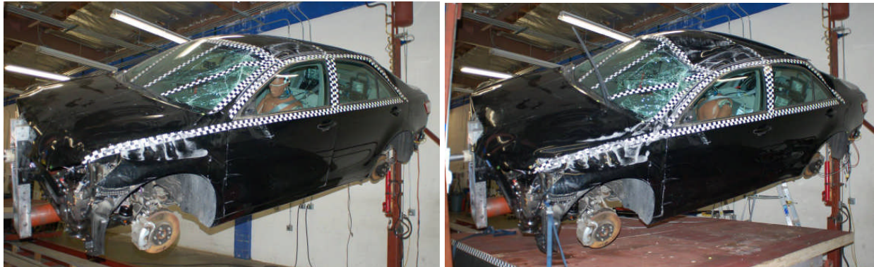
Figure 4. The 2007 Toyota Camry after the first roll JRS test (left) and the second.
