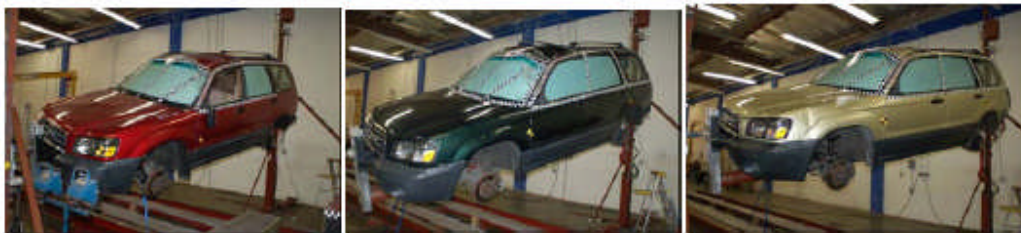
Photo of three Subaru Foresters used for repeatability testing, courtesy of Center for Injury Research
