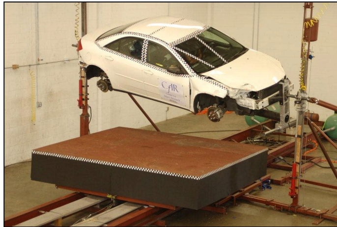
Photo of JRS test device, courtesy of the Center for Injury Research
