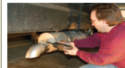
The combination of Diesel Particulate Filters (DPFs) and Ultra-Low Sulfur Diesel (ULSD) can achieve a 90% reduction in diesel particles.
