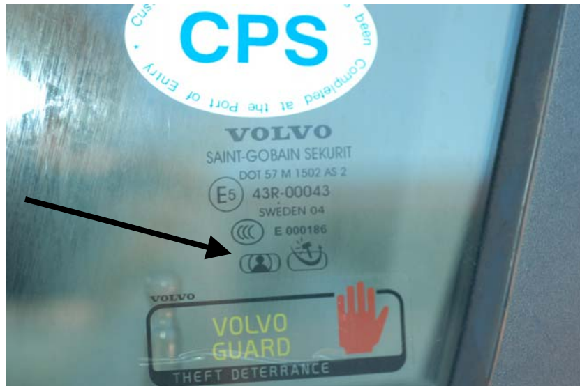
2004 Volvo S80 side glazing – monogram indicates occupant protection capability (left) and added security against “smash and grab” robberies (right).
